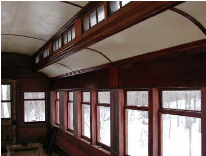
You can begin to see the luster of the mahogany come out as the varnish is applied. Contrast the unvarnished wood. David Woodbury photo.
